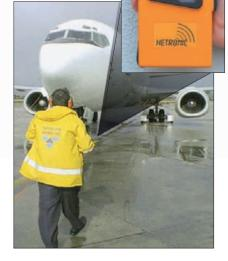
Simple one-man remote control The driver's position is unmanned during pushback. A simple handset allows easy remote control with wingtip to wingtip visibility.
