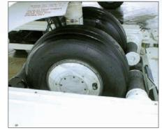
No forces are exerted on the landing gear structure, nor is the aircraft lifted from the ground.
