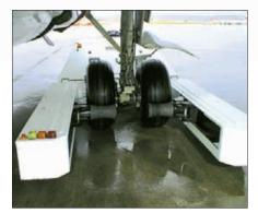
...pressure rollers grip the tyres. Rotational friction forces drive the aircraft's wheels.
