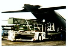
Able to handle aircraft with door sill heights of up to 3.450 mm, the SCHOPF HC100 loader/transporter demonstrates its advantages as a transfer link between aircraft/aircraft, aircraft/dollies, loaders/dollies as well as direct truck transfer.
