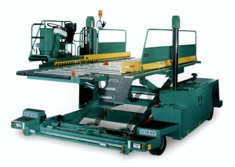
Even bulky and oversized cargo can be handled easily by the SCHOPF HC100 loader/transporter
