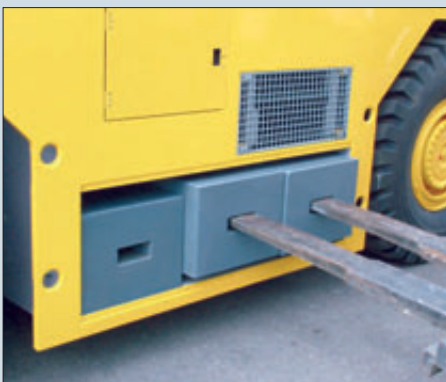
Quick and easy ballast removal enables tractor weights between 50 - 70t
