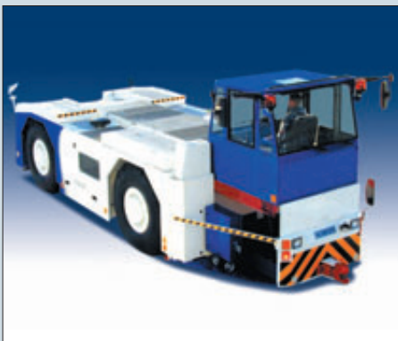
High-lift driver's cab with turntable seat for safe operations in forward or reverse
