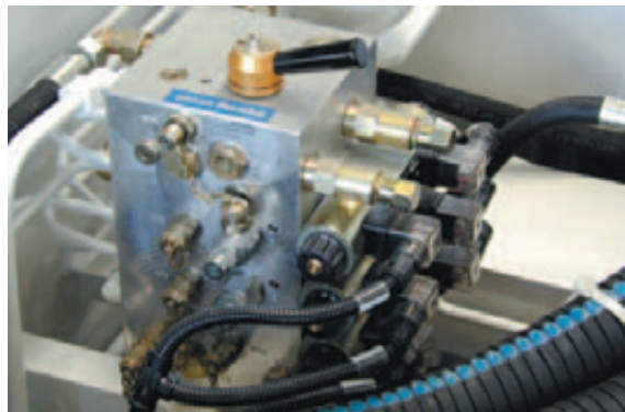
Minimess® hydraulic test ports – for thorough system checks
